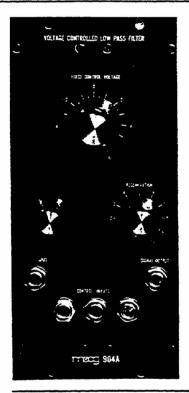
Figure 4.10A. Moog 904A Low Pass Filter
